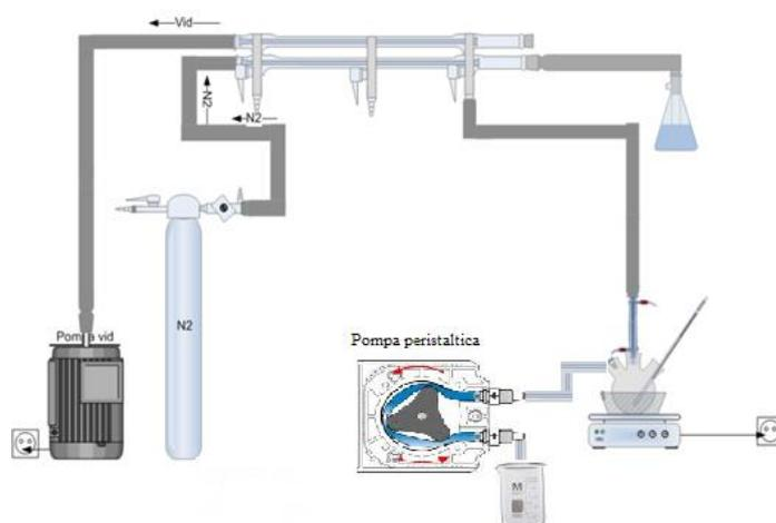
Figure 1. The experimental installation used for synthesis
