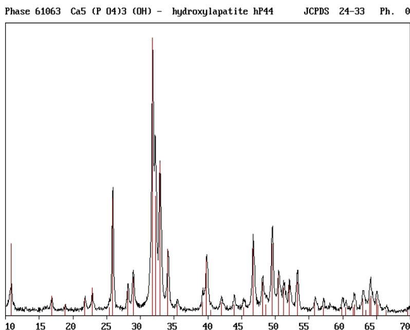
Figure 2. Diffraction spectrum of synthesized hydroxyapatite and position of the peaks corresponding to the commercial HA (red) from the database JCPDS
