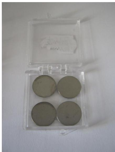
Figure 5. Titanium metal discs coated with a HA-AL 20 mM microfilm by MAPLE
