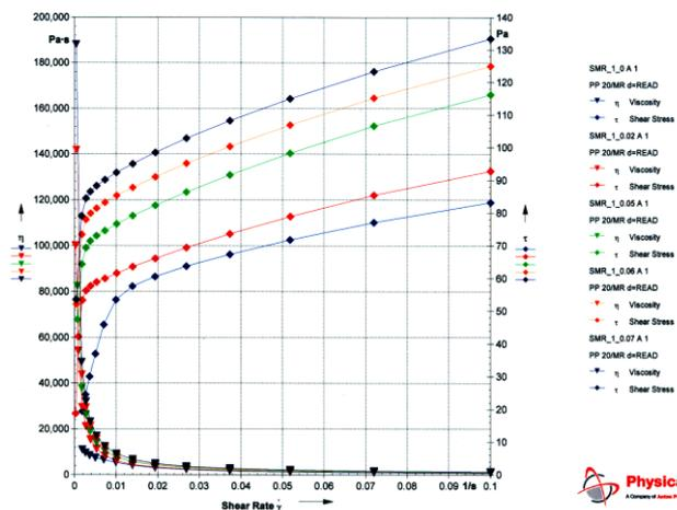
Figure 103. The rheological properties of the suspensions were determined with the MRD 180 (Physica 9 type) re-viscometer
