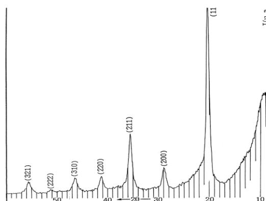
Figure 87. The röntgenogram of the magnetorheological suspension based on silicone oil, stearic acid and iron microparticles
