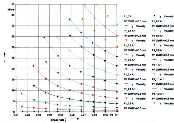
Figure 104. The rheological properties of the suspensions were determined with the MRD 80 (Physica 9 type) re-viscometer
